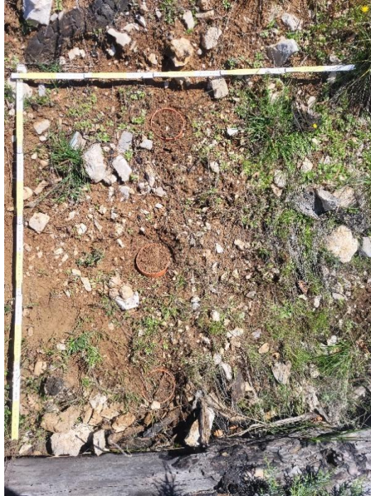
Figure 20 PVC collars (10 cm diameter, 5 cm depth) installed at the study sites to measure soil CO 2 Efflux using the closed-chamber method. Collars were left in place for at least two weeks before data collection to allow soil stabilization.
