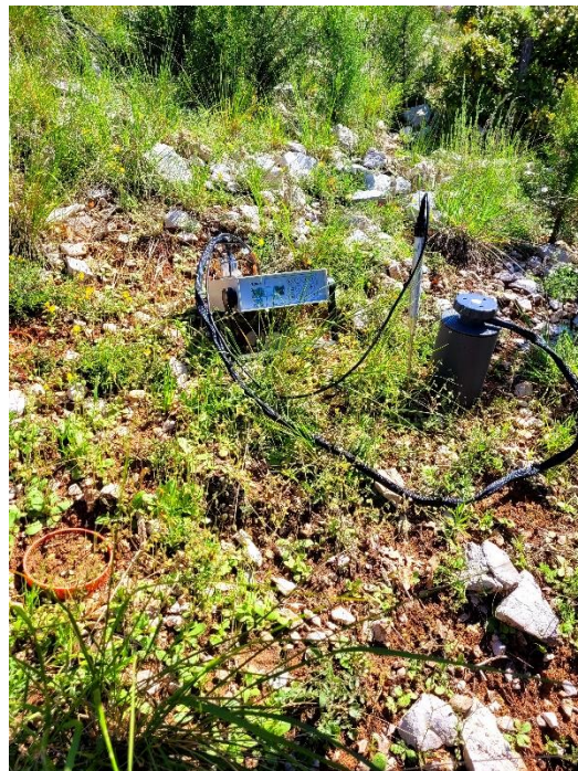
Figure 21 Portable infrared gas analyzer (EGM-4, PP Systems) connected to SRC-1 closed chamber, used to measure soil CO 2 Efflux at each collar.
