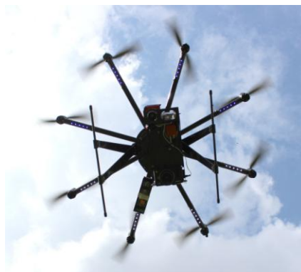
Figure 3.2 - octocopter UAV, Aerialtronics Altura AT8 v1A equipped with all essential tools
