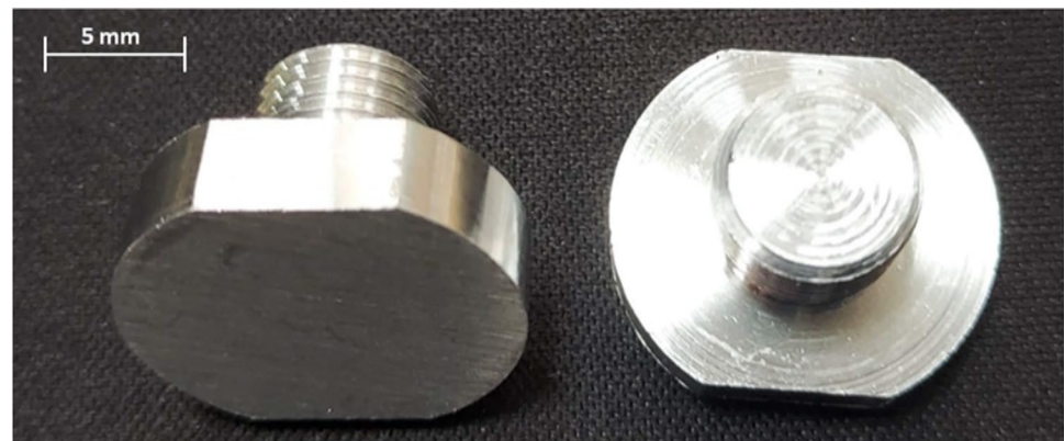
Fig. 1 Samples made according to ASTM-G32-10 standard [40]
