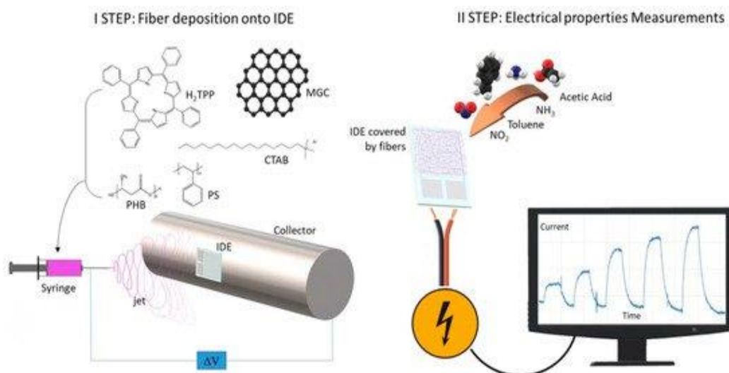
Figure 5.3. Sensor developing and usage scheme. The polymer mixture loaded in the syringe ( Left ) was electrospun by applying a voltage between the tip and the cylindrical collector where an interdigitated electrode is fixed and coated with the fibers. The coated IDE was used as transducer ( Right ) and connected to a PC for sensing current changes upon interaction with gases molecules.
