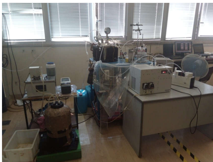
Figure 3. Hybrid gas-stirred tank reactor (GSTR) employed in the experiment.
