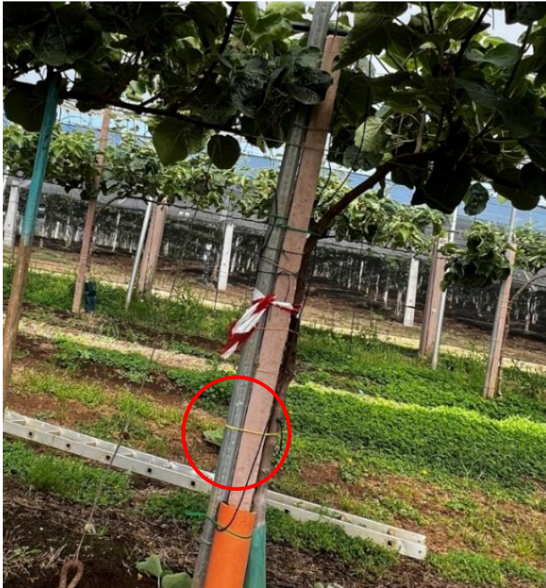
Figure 1.2. Sap flow probe of Tree Talker (TT) system in action at Tre Colli S.r.l, located in Cisterna di Campoleone (Velletri, Rome, Italy)
