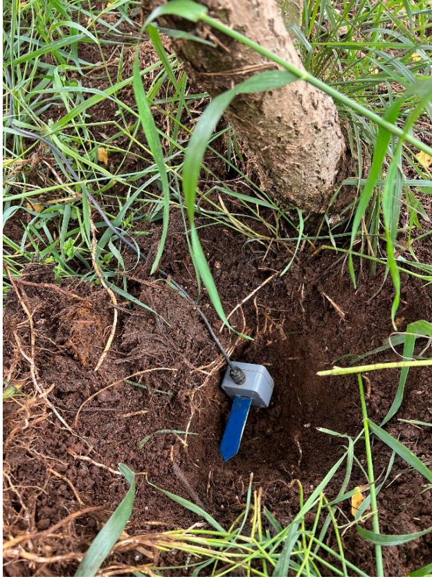
Figure 1.4. Soil moisture sensor placed 30 cm underground at root system level of ‘Soreli’ kiwi plants located in Tre Colli S.r.l, located in Cisterna di Campoleone (Velletri, Rome, Italy)
