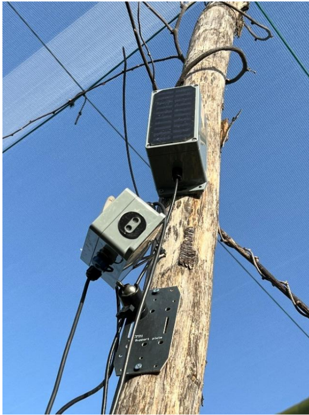
Figure 1.3. Kiwi plant leaves monitored by TT device equipped with spectrophotometer with 12 spectral bands Tre Colli S.r.l, located in Cisterna di Campoleone (Velletri, Rome, Italy)
