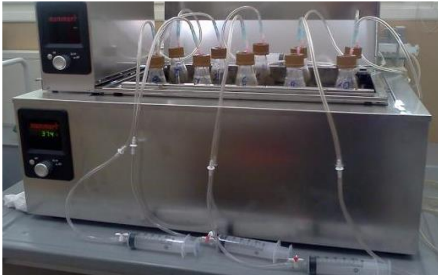
Figure 1 - Experimental configuration for batch anaerobic digestion
