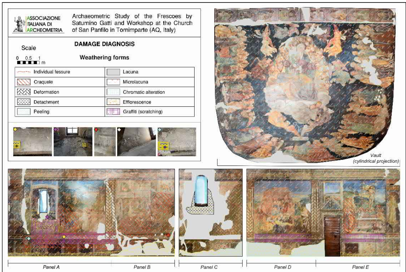
Figure 9. Distribution of the weathering forms affecting the five panels and the vault of the apsidal conch of St. Panfilo Church in Tornimparte (AQ, Italy). Coloured dots indicate the position of the acquired pictures in the wall paintings.
