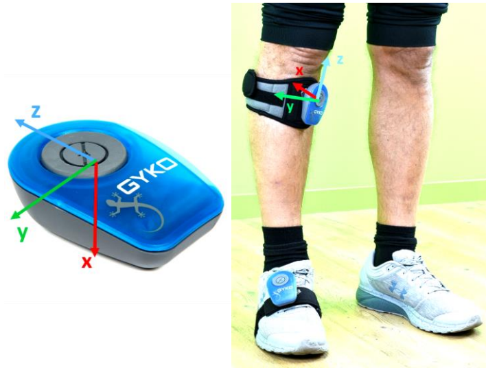
Figure 23. MIMU placement: ad hoc straps and tape were used to fix MIMUs on the foot and tibia.
