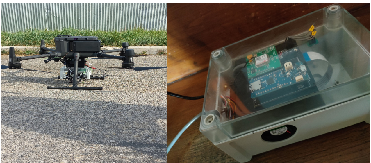
Figure 40 Gas analyzer mounted below a drone and close-up of the device
