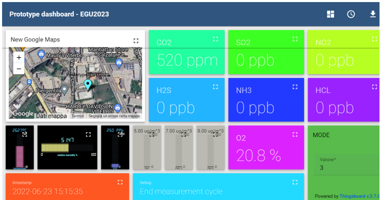
Figure 39 Example of a Thingsboard dashboard for a gas analyzed prepared for the presentation of the device at EGU23
