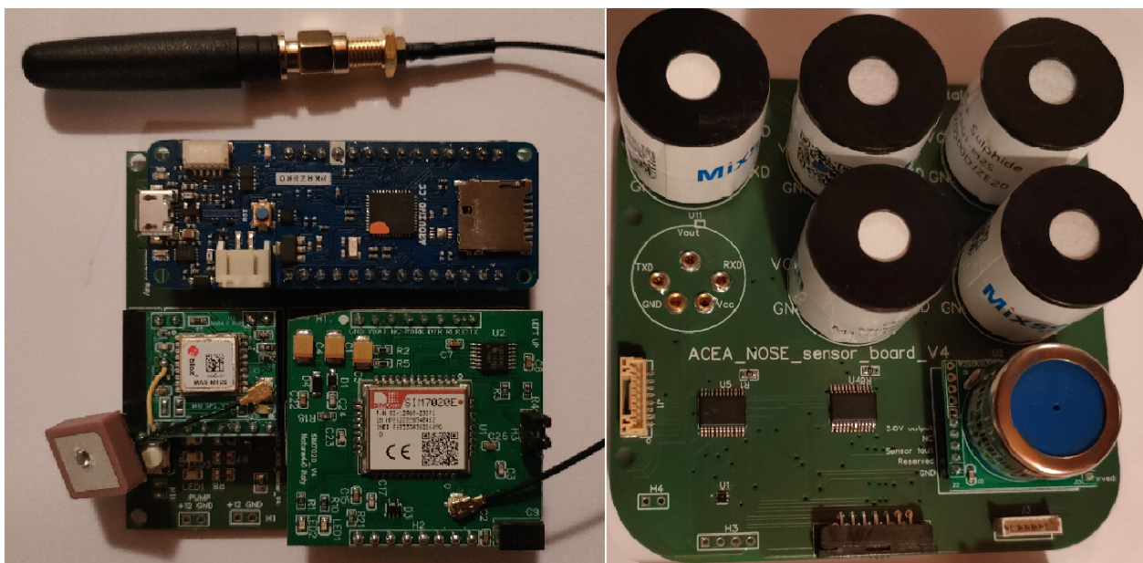
Figure 36 On the right the control board and on the left the sensor board with six electrochemical sensors inserted
