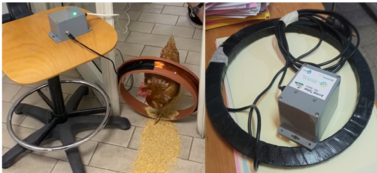
Figure 34 Experiment performed on an RFID tag injected in the chicken and on the right the final version of the RFID reader. Thanks to the “Istituto Zooprofilattico Sperimentale del Lazio e della Toscana M. Aleandri” in Viterbo and Dr. Erminia Sezzi for her valuable assistance and suggestions during the experiment.
