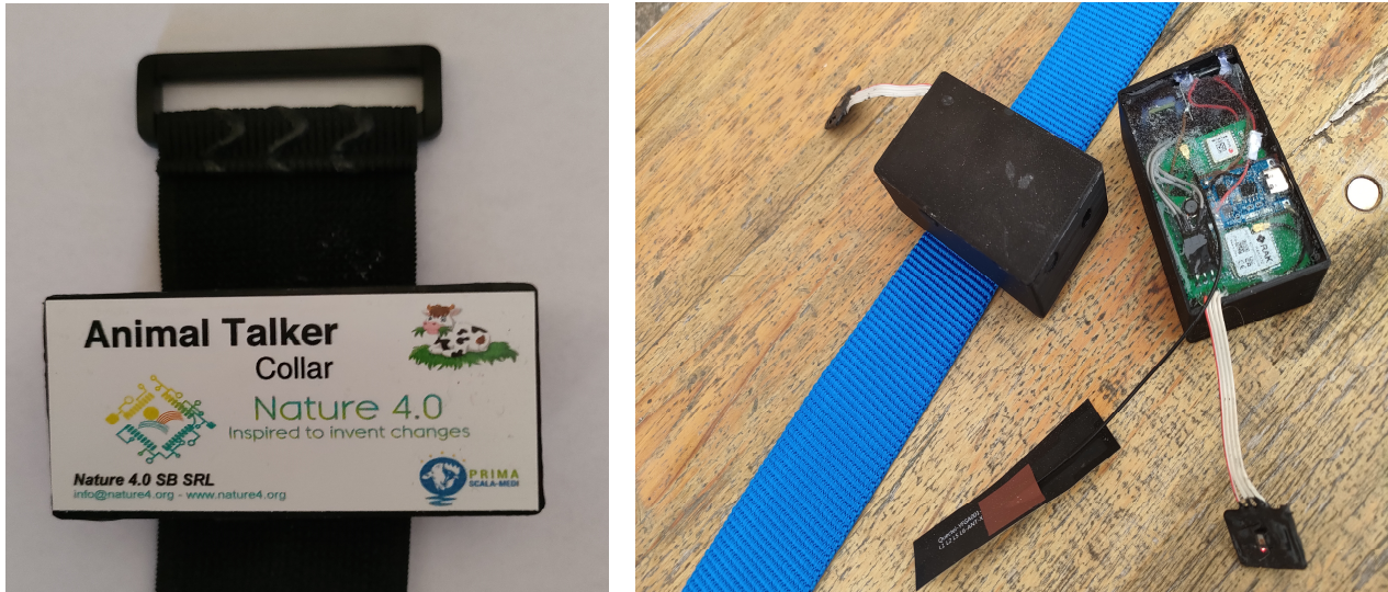
Figure 17 On the right the ovine version of the animal collar devices is shown, on the left the one for bovine. The opened box allows to see the antenna, the switched on heart rate sensor and some components such as the USB charger, the LoRaWAN module, the GNSS module and the magnetic switch. The box is filled insulant electronic gel.
