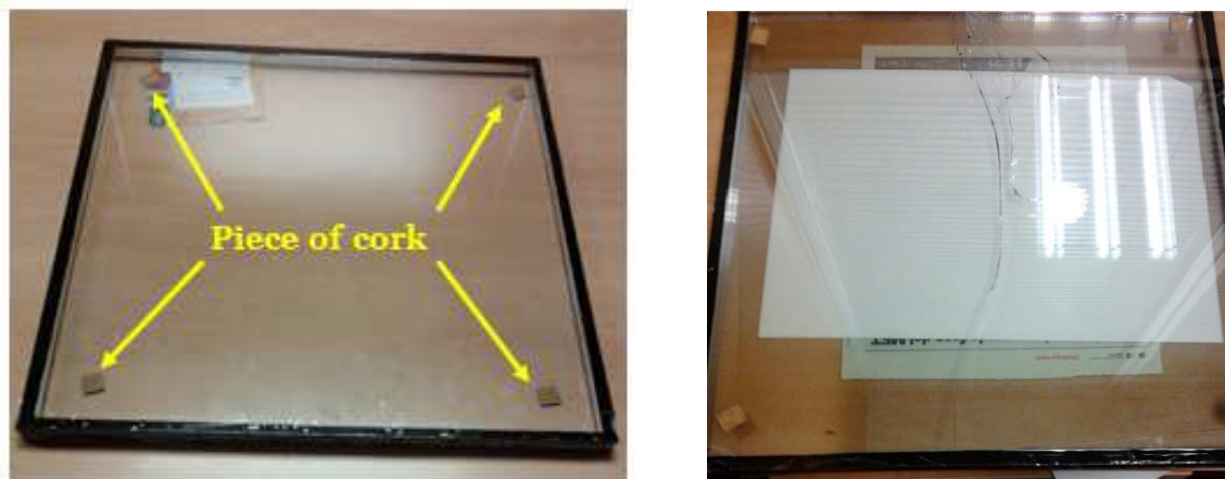
Figure 66: Side "a" and "b" of the glass (left) and glass 2 after breaking (right).
