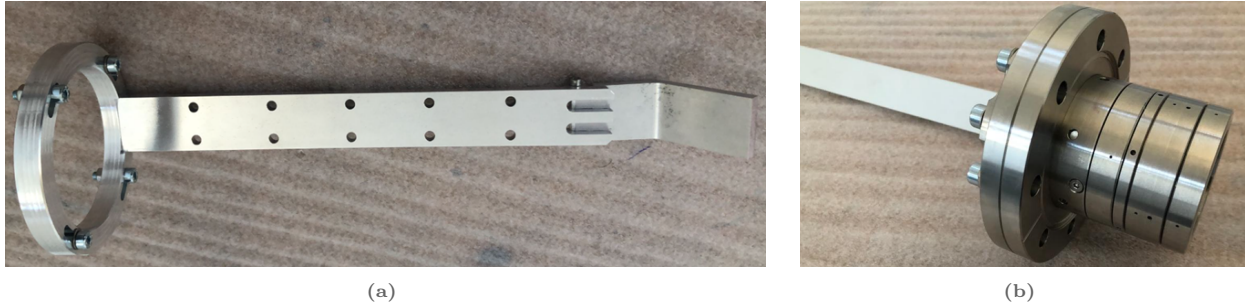
Fig. 20.4: Picture of the components: (a) support for the flat mirror installed inside the spherical vessel; (b) lenses holder and CF-63 viewport
