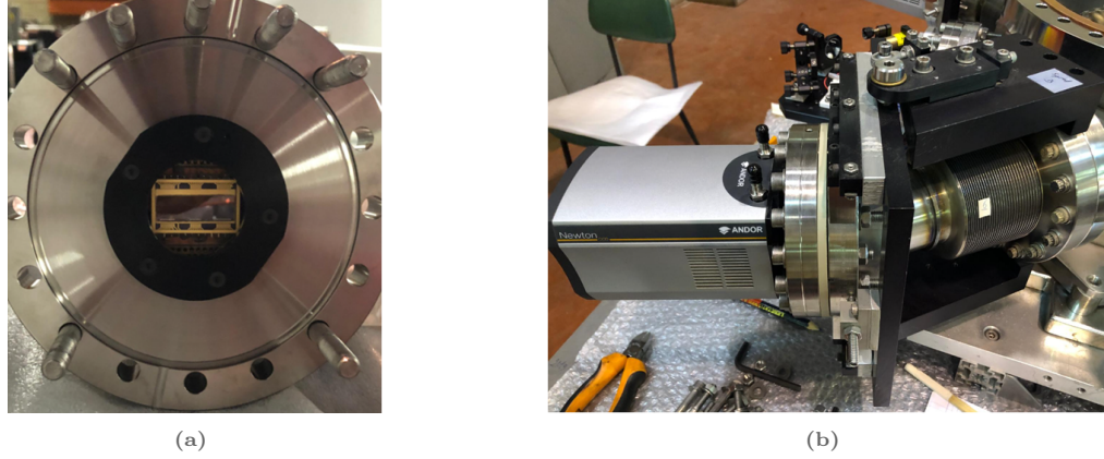
Fig. 19.17: CCD installation: (a) picture of the CCD sensor; (b) picture of the CCD installed. The peek insulator between the camera and the bellow can be seen (light brown).
