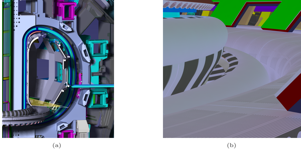
Fig. 7.4: Simulation of the possible view of the imaging spectroscopy system from port 4: (a) field of view; (b) image simulated.
