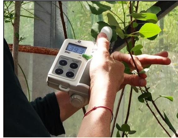
Figure 6 Chlorophyll content measurement with SPAD
