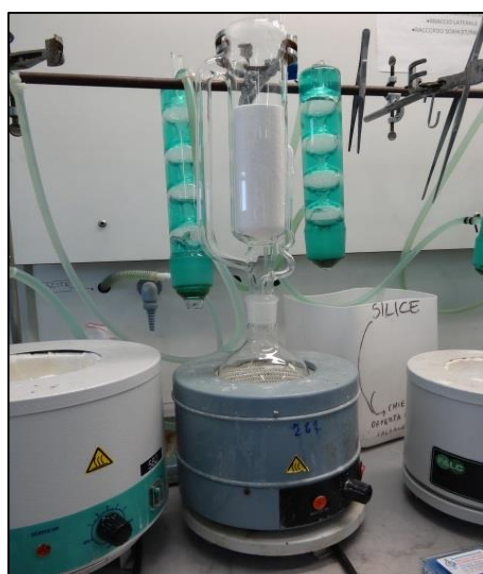
Figure 3 Soxhlet extraction. laboratories of the institute of atmospheric pollution research , IIA-CNR (Rome).
