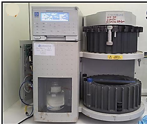
Figure 5 Accelerate solvent extraction (ASE 200, Dionex), laboratories of the institute of atmospheric pollution research , IIA-CNR (Rome)
