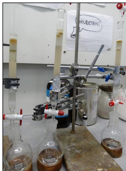
Figure 8 Silica \text{H}_2\text{SO}_4 clean-up, laboratories of the institute of atmospheric pollution research, IIA-CNR (Rome)
