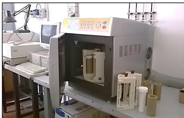
Figure 4 Microwave extraction system (Excel , EU Microwave Chemistry Technology Instruments Co.), laboratories of the Institute of agro-environmental and forest biology, IBAF-CNR (Rome).
