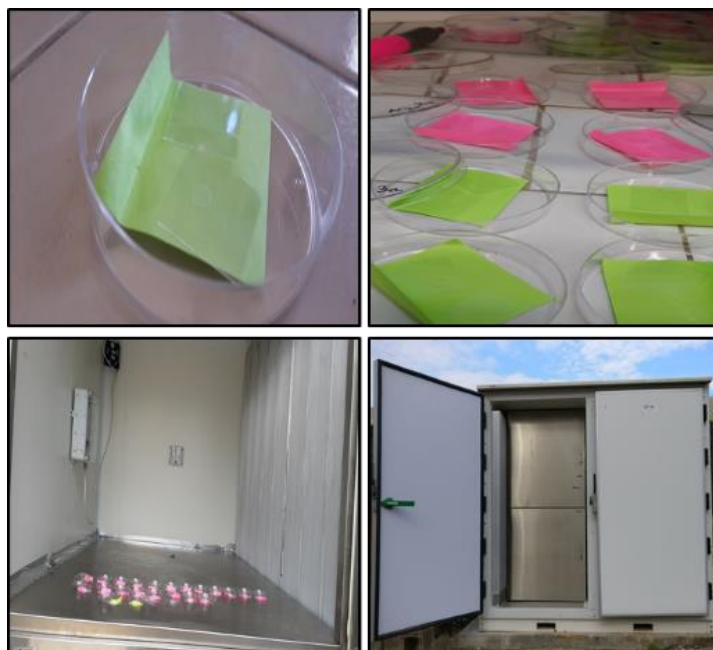
Figure IV-2: AfB1 and OTA distributed on glass slides and treated with ozone at 0.1, 0.3 and 2ppm for 5 or 10hours. Three replicates were used for each combination.
