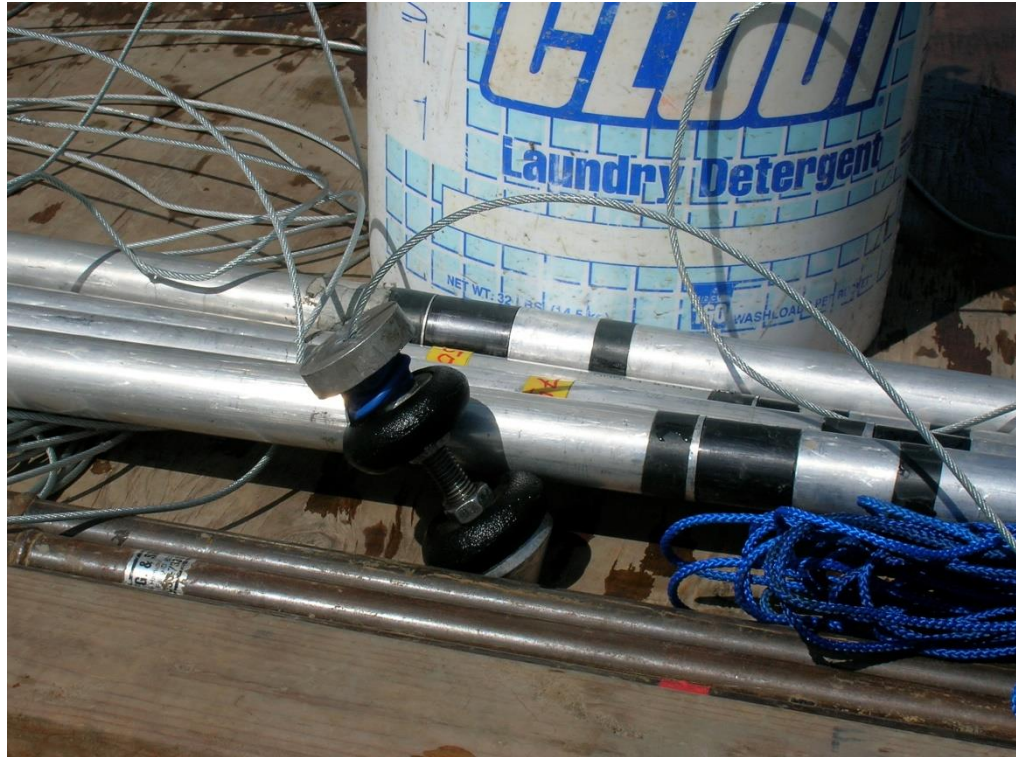
Figure 2 – The modified square rod Livingstone hand operated corer
