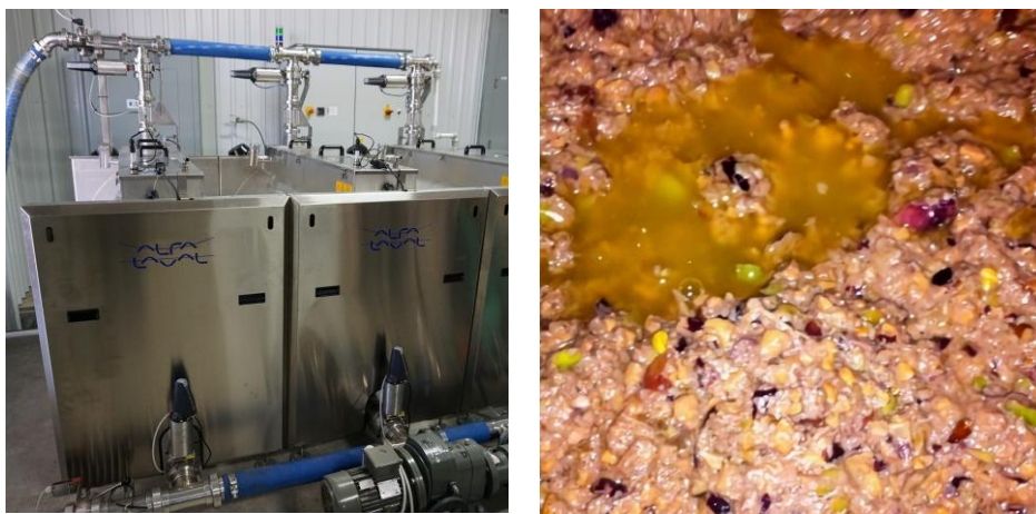
Figure 1. A malaxer (on the left) (Clark, 2016); olive oil droplets coalescence during OP malaxation (on the right) (OKelly, 2010)
