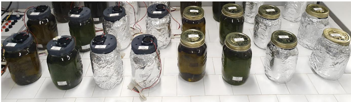
Figure 1. Experimental setup illustrating different treatment combinations applied to olive oil samples. Conditions include air exposure (fans on jars), light exposure (clear versus foil-wrapped jars), and thermal stress (brown colored oil).
