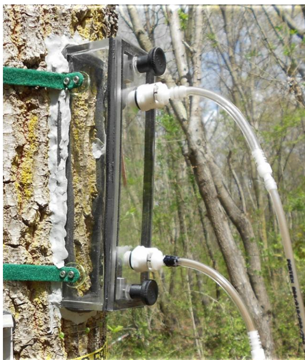
Fig. 2.4 – Chamber with a fixed collar on the stem to 1.30 and a removable lid connected to a portable infrared gas analyzer by flexible tubing.
