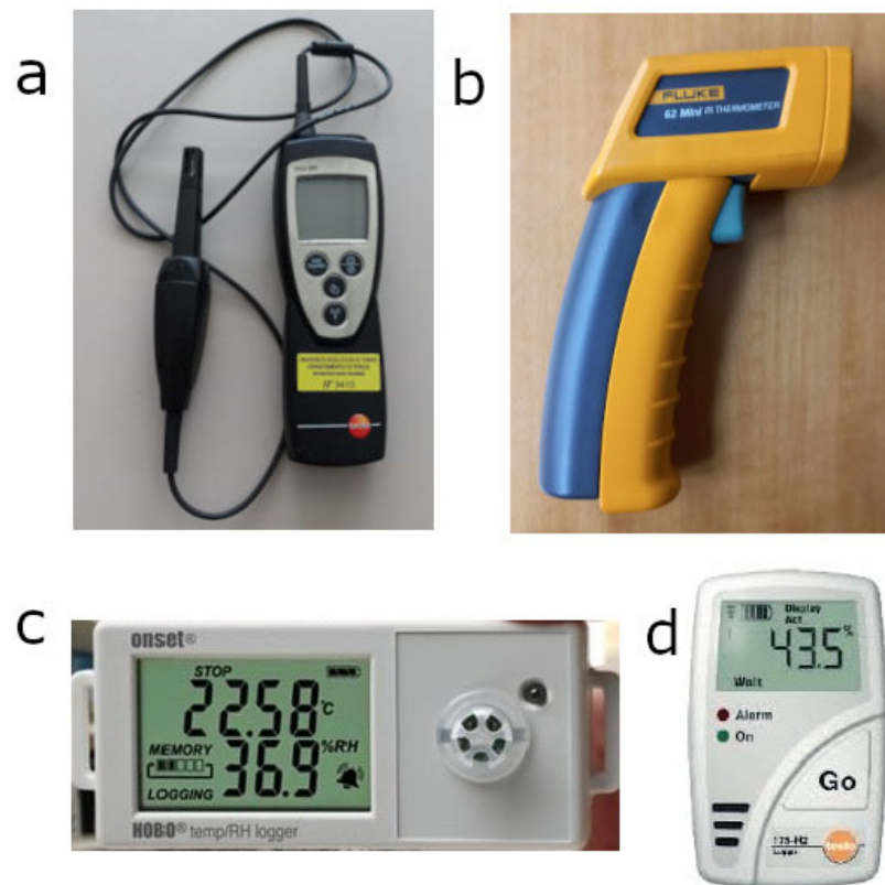
Figure 3. Instruments: (a) Testo 625 thermo-hygrometer, (b) Fluke 62 Mini infrared thermometer, (c) HOBO-UH100-011 thermo-hygrometer, and (d) Testo 175-H2 thermo-hygrometer.
