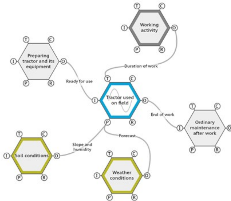
Figure 38: basic FRAM model for safety-related functions involved in tractor usage which can affect rollover probabilities
