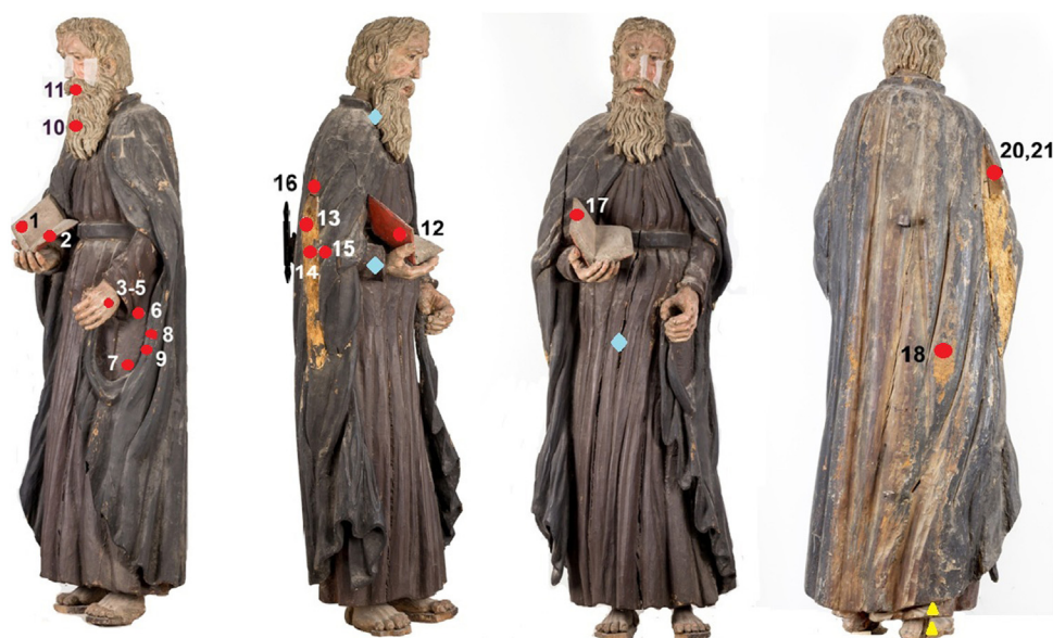
Fig. 2. Different views of the sculpture. In red the points examined by means of XRF analysis, in yellow the points selected for stratigraphic analysis, in light blue the points sampled for wood microscopic analysis. (For interpretation of the references to colour in this figure legend, the reader is referred to the web version of this article).
