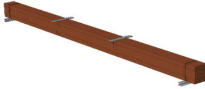
Fig. 11. a) Four-point bending experimental setup, b) FE model beam with ending support and load plates details c) Setup carriage, d) Setup hinge.
