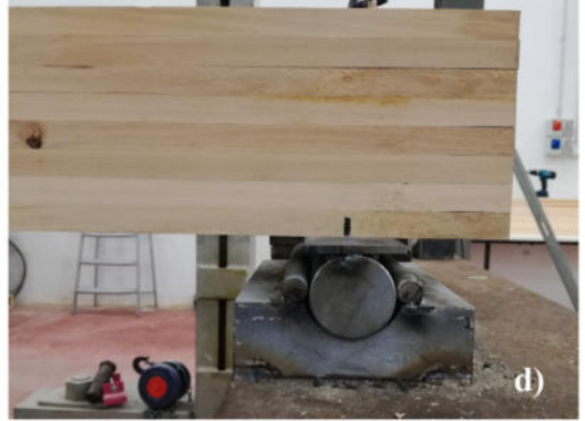
Fig. 11. a) Four-point bending experimental setup, b) FE model beam with ending support and load plates details c) Setup carriage, d) Setup hinge.
