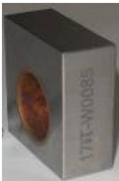
Figure 3.1: W monoblock with Cu interlayer
