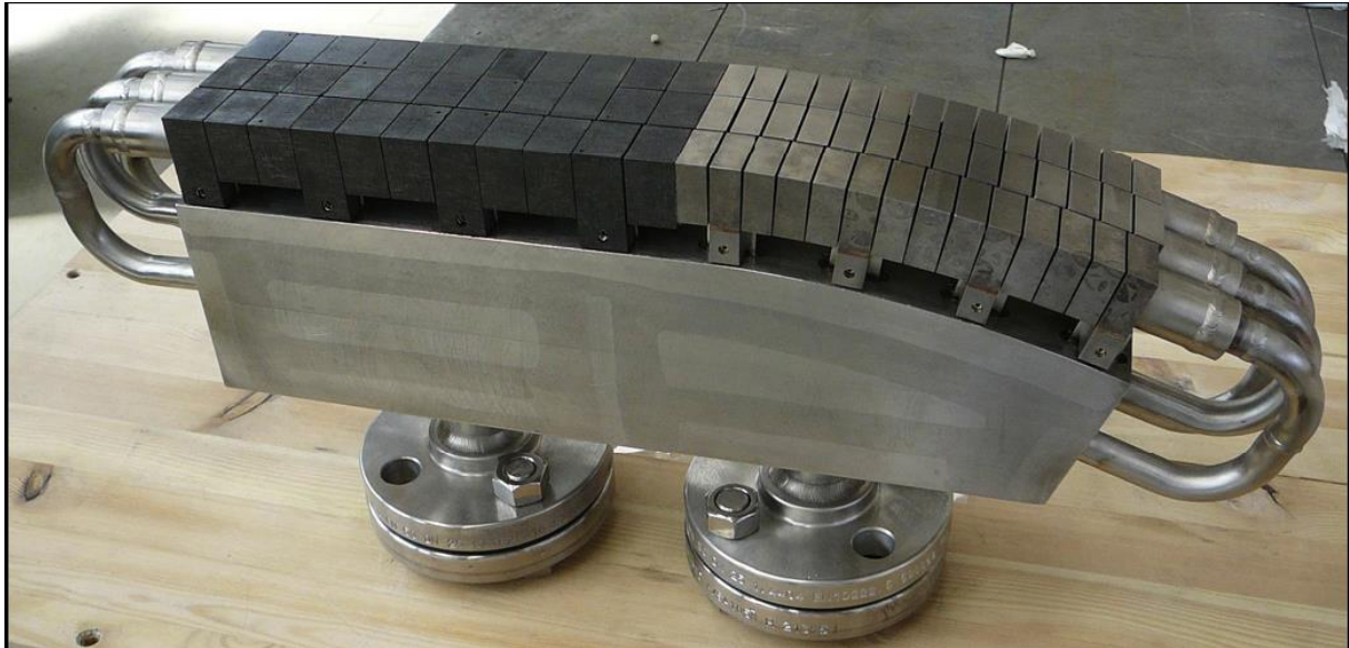
Figure 2.2: Small scale prototype of plasma facing component with straight part in Carbon Fiber Composite
