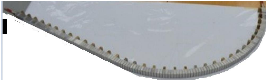
Figure 3.3: The full-scale full W PFU after HRP
