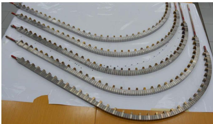
Figure 2.10: Full-scale tungsten IVT PFUs
