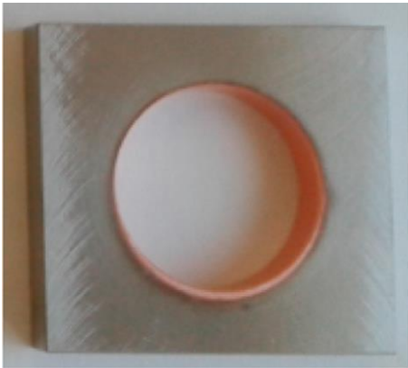
Figure 2.8: tungsten monoblock with a hole before joining to a tube. The inner wall was coated with a graded W/Cu bond coat
