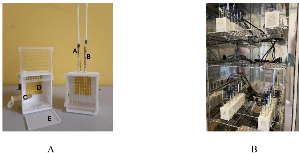
Figure 3.3. A) Self-built 3D printed cages used for trials with SS50 (1), tap water (2), protein diet (3), wax foundation (4) and removable try (5). B) Setup of the incubator during the test. (Author's photos).
