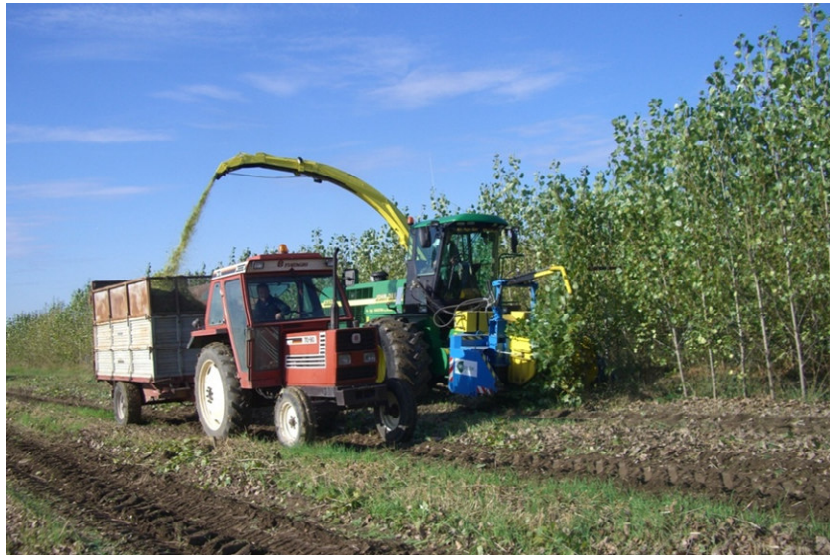
Figure 4. Harvesting of two years poplar SRF by modified forage harvester.
