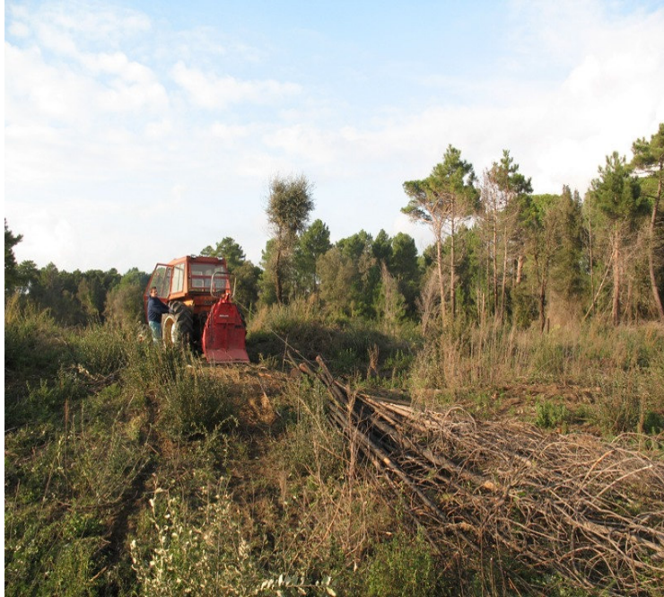
Figure 2: Whole tree winching operated by farm tractor equipped with forest winch
