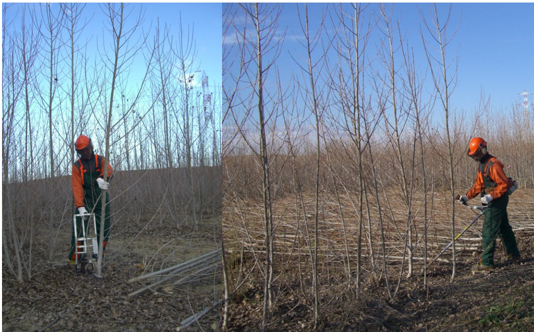
Figure 1: Felling of two years poplar trees by chainsaw with felling frame (on the left) and cleaning saw (on the right).
