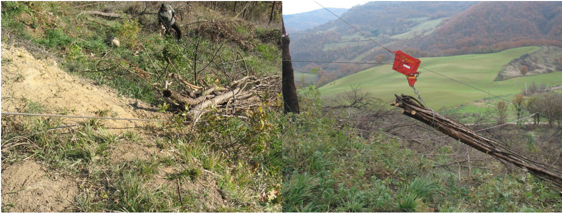
Figure 2: Comparison of winching (on the left) and small cable yarder extraction (on the right).
