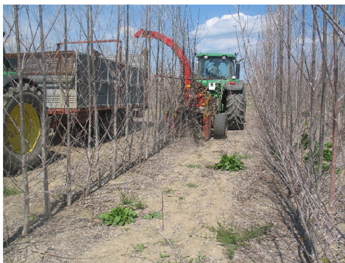
Figure 3: Harvesting of poplar two years SRF by tractor driven harvester-chipper head.
