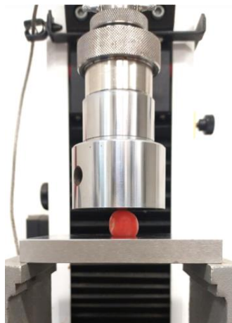
Figure 3.5. Firmness measurement by Instron® Universal Testing Machine.
