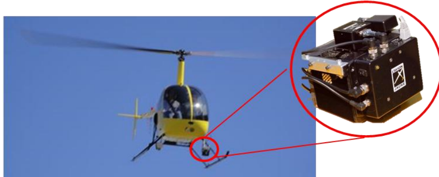
Figure10:LiDAR sensor mounted on a small ultra-light helicopter, used for this study..
