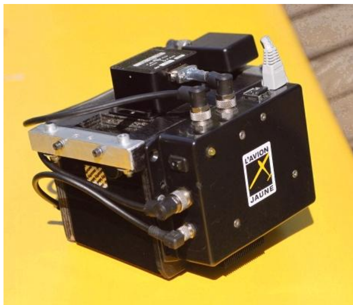
Figure 9: Prototype of LiDAR sensor mounted on lightweight platform.
