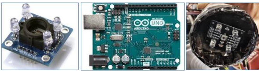
Figure 1: the TCS3200 sensor (on the left) and the Arduino UNO board it was connected to (in the centre) and detail of the colour sensor inside the aluminium-coated plastic shield (on the right).
