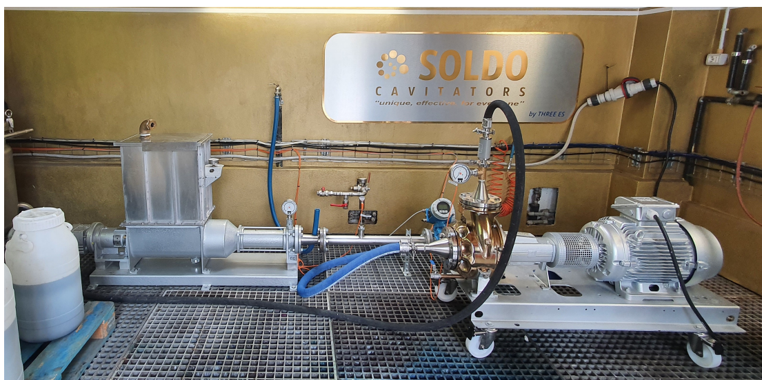
Figure 3.2: Cavitation unit patented by SOLD0 Cavitors [15].
