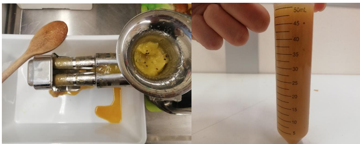
Figure 2.2. Extraction process of the Soreli's juice-by Electric Juice Extractor, Mod. 7500 Angel Co.Ltd.
