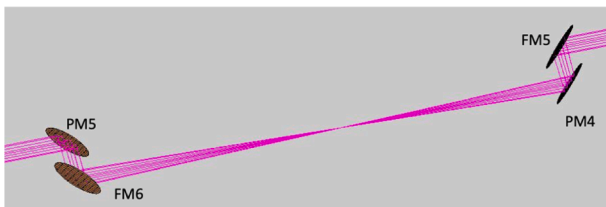
Fig. 10. section of the original MB TL between FM5 and PM5 with the beam axes of the 9-mirror crossing between PM4 and FM6.
