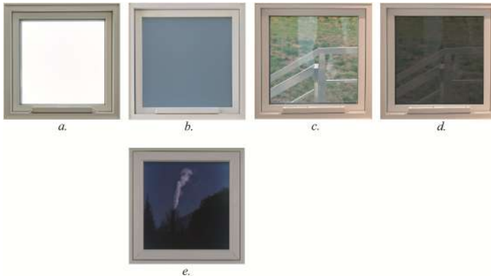
Fig. 15. Basic combinations of window states: frames a , b , c , d are window views from the house interior, while frame e is a view of a fully tinted window from the house exterior.
