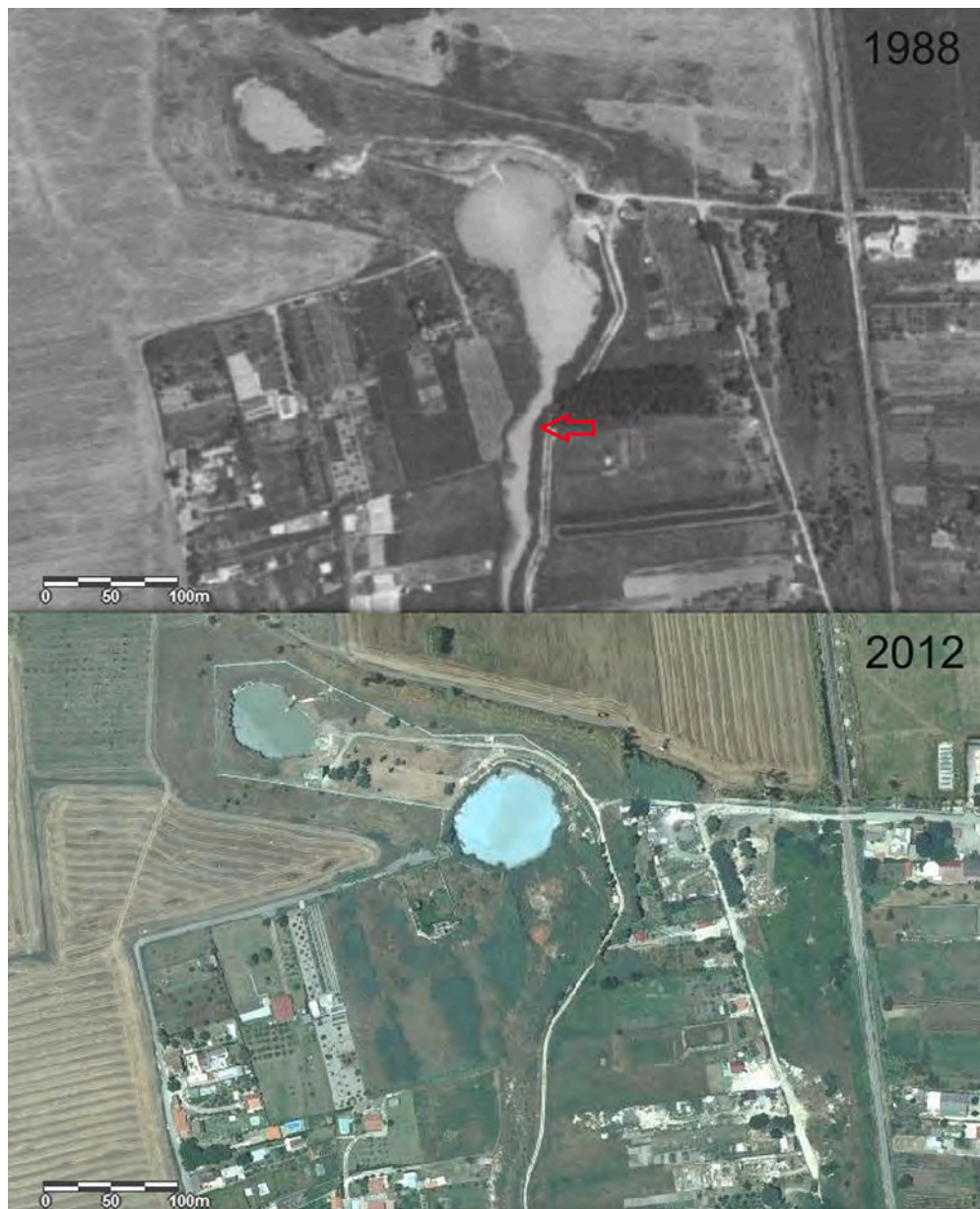
Fig. 2. Comparison of the 1988 and 2012 orthophotos of the area of the Acque Albule springs, showing the reduction in size of the discharge zone and the absence of natural groundwater outflow (highlighted by the red arrow in the 1988 picture) from the springs in 2012 (Geoportale, 2023).
