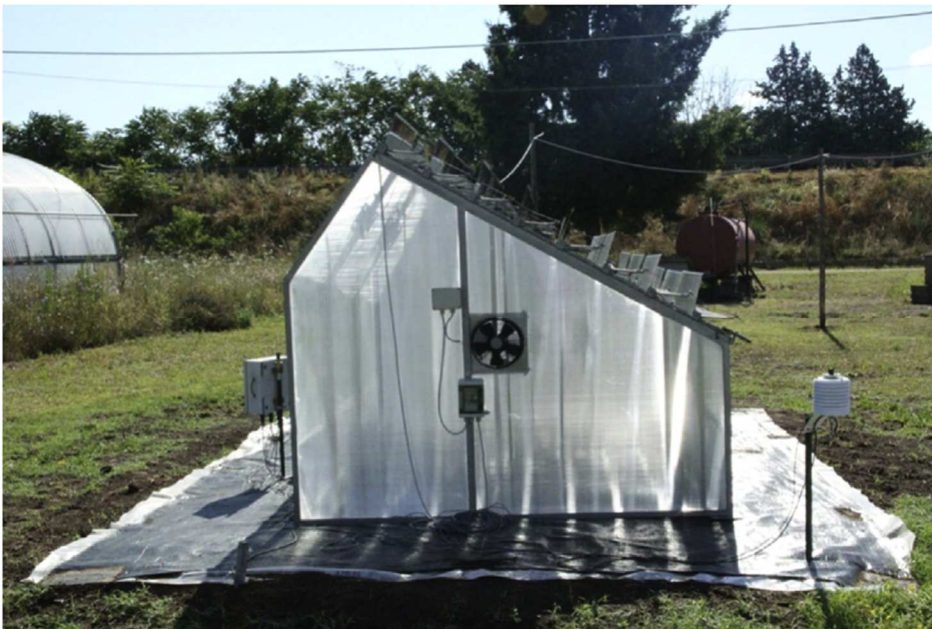
Fig. 1. Asymmetrical cross section of a prototype dynamic photovoltaic greenhouse.
