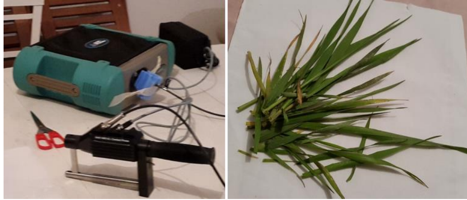
Figure 6. Hyperspectral acquisition system. On the left side are shown the tools used for hyperspectral data acquisition; on the right is shown an example of wheat leaves sample.
