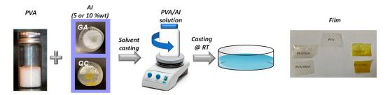
Scheme 1. Procedure for the preparation of poly(vinyl alcohol) (PVA) formulations.
