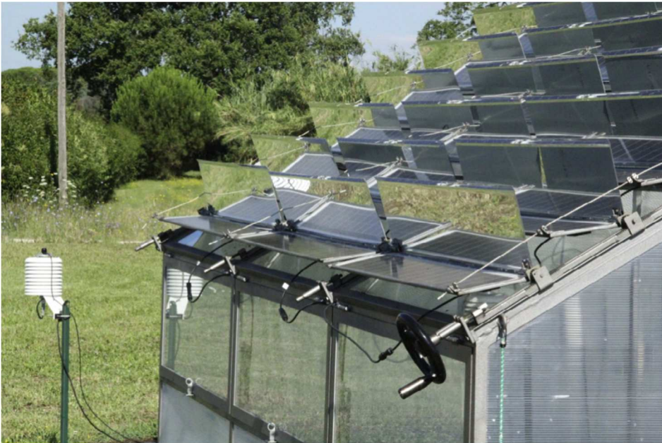
Fig. 5. Movement system of the photovoltaic panels and highly reflective aluminum mirrors.
