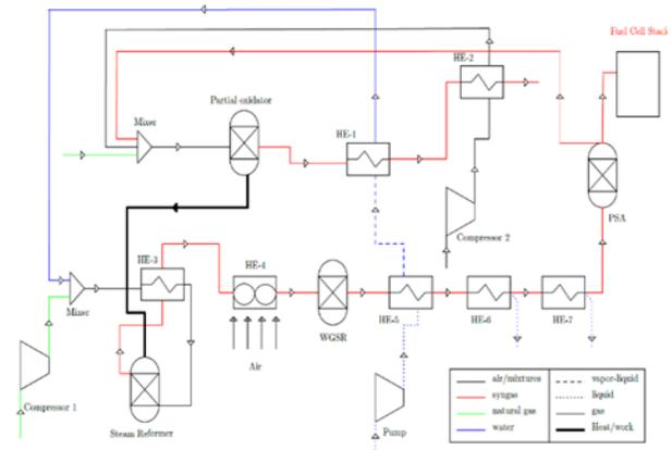
Fig 4: Schematic of the CHP plant concept: energy system
