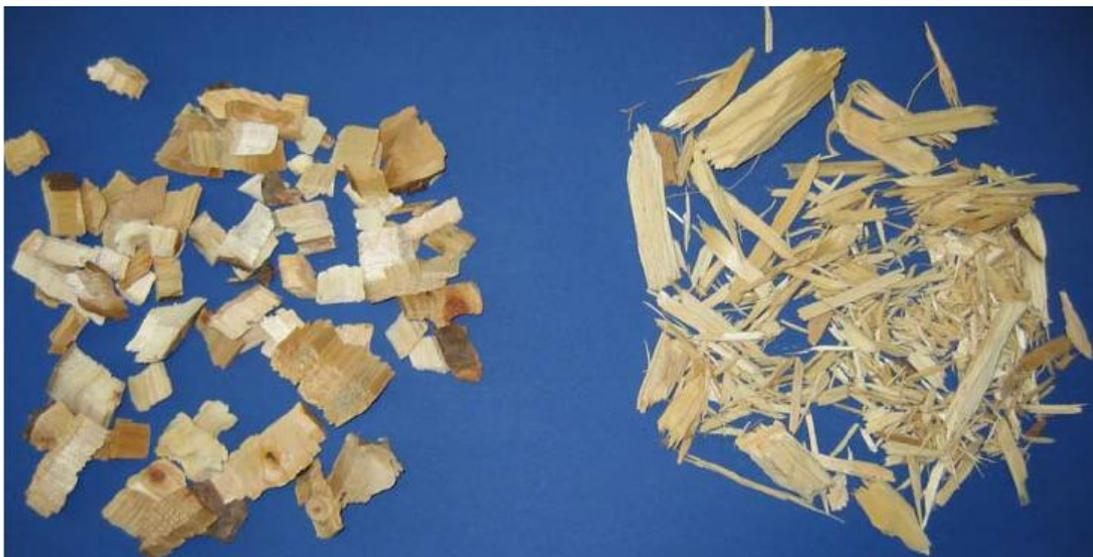
Figure 3 - Visual differences between wood chip (left) and hog fuel (right).
