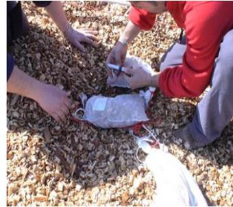
Figure 8 - Installation of samples and thermocouple in a measurement point.
