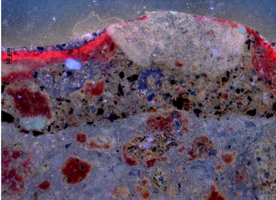
Fig. 2 – Thin section of a micro sample taken from the red area on the right of the mosaic (red false mosaic reintegration).
