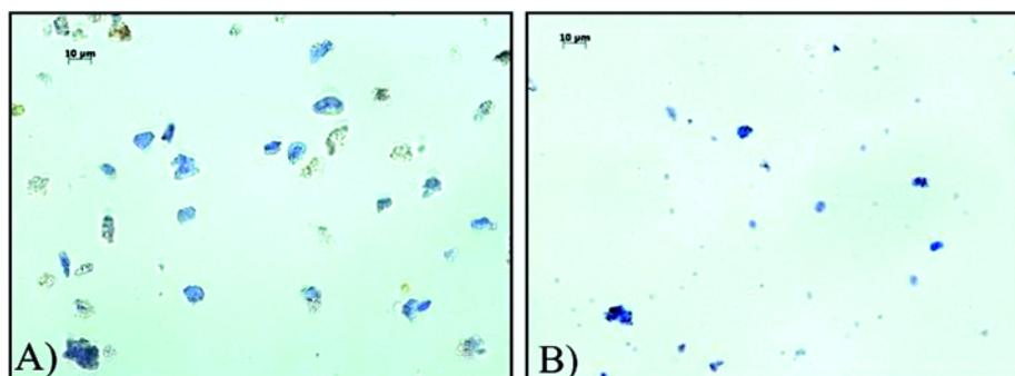
Fig. 3 – Photomicrographs of the blue pigments. A) 1950 false mosaic integration, cobalt blue; B) 1975-1980 additional touches on the mosaic surface, artificial ultramarine. Transmitted light, N//, ob. 40x.
