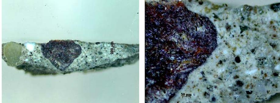
Fig. 6 – Cross sections at two different magnifications of the hard cementitious mortar.
