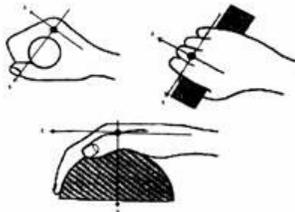
**Figure 1. Definition of the measurement axes (ISO 5349)**
